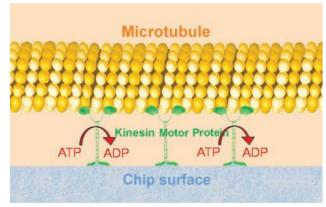
power microfluidic motors based on kinesin – a protein that moves as it hydrolyses ATP. Currently, ATP is produced in microfluidics with the enzyme pyruvate kinase, but this is a low energy density fuel, and an improved ATP source is the goal.
