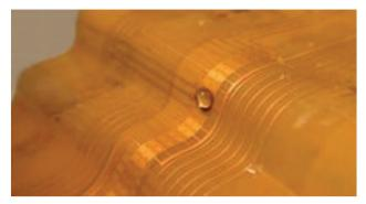
of the droplet. This process gives the team full control of the droplet, including up and down vertical surfaces.
