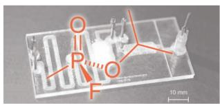
The blood flows through the chip in a sequence of steps. Initially, the blood cells are burst open and the sarin released, before the blood proteins and other particulates are filtered out. The purified mixture is then mixed with a substrate and a chromophore, and passed over an immobilised enzyme. If the sample contains no sarin, the enzyme reacts with the substrate, which then attacks the chromophore, which is detected by an external UVvisible spectrometer. But if sarin is
